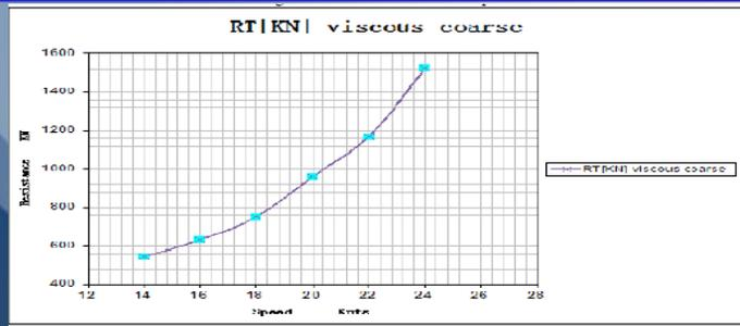
Figure 25. Ship resistance for Viscous flow.
