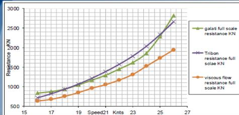
Figure 27. Comparison results for KCS full scale test with Tribon and viscous flow results.
